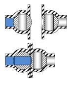
Both ball valves are locked in closed position. The engaging mechanism prevents them from being turned
