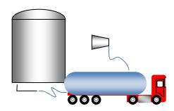
The liquid will flow to the tank powered by the pressure of the air or gas flowing from the compressor.
