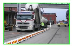
There must be free egress from the loading/ unloading area. If the truck driver has inadequate visibility when coming onto a public road, he must be assisted by an operator.
