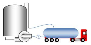
The pump will be filled with liquid by gravity and will provide the necessary energy to the product to overcome the gravitational backpressure and flow restrictions. The pump will be connected to the vehicle by a flexible hose of sufficient diameter (usually 80mm -3"). The liquid flowing will simultaneously create more vapour-space in the vehicle and less in the site tank. A flexible hose (minimum 50mm - 2") connecting both vapour-spaces will balance the pressure and prevent
