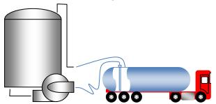
The same possibilities exist as for bottom discharge except that – since access to the top of the vehicle is already required for connecting the liquid-hose. Having to access the top of the vehicle for connecting or opening the vapour connection is no longer a disadvantage. (Provided of course the site has taken the relevant working at height precautions)
