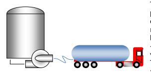
The pump will be filled with liquid by gravity and will provide the necessary energy to the product to overcome the gravitational backpressure and flow restrictions. The pump will be connected to the vehicle by a flexible hose of sufficient diameter (usually 80mm -3"). The liquid flowing will simultaneously create more vapour-space in the vehicle and less in the site tank. The Site tank's vapour will exit the tank to the atmosphere (possibly through a scrubber or Vapour-
